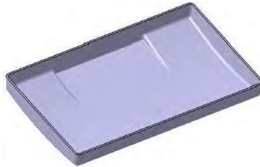
Figure 5-101 Resulting shelled model
