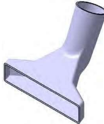
Figure 5-86 Final model after shelling
